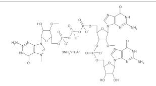
Using the conditions described here, transcription with CleanCap GG and CleanCap GG (3' OMe) results in 70-90%<sup>1</sup> capped material, generating a Cap 1 structure and gives crude yields of ~1.5 mg per mL of transcription.
